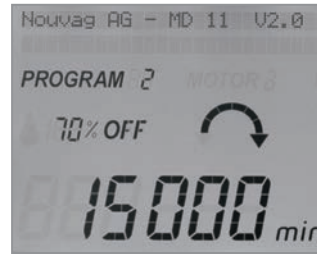
Set Your Motor To 12,000-15,000 RPM Translates To 120-150 Gentle Taps Per Minute (Max 15,000 RPM)
